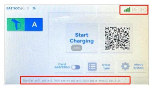
B. After the charging gun is connected to the electric vehicle, the user starts charging through the OCPP background/mobile APP, and waits until the system starts charging, as shown in the following figure:
