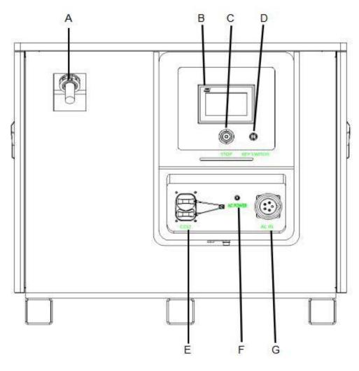
Energy storage battery system-front panel
