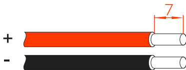
Figure3-16 Stripping diagram of DC input (unit: mm)
