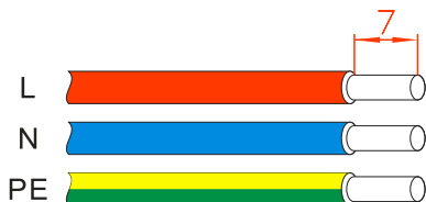
Figure3-21 Stripping diagram of AC output (unit: mm)
