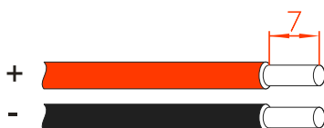
Figure3-14 Stripping diagram of DC input (unit: mm)
