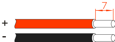
Figure3-16 Stripping diagram of DC input (unit: mm)
