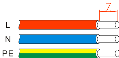
Figure3-21 Stripping diagram of AC output (unit: mm)
