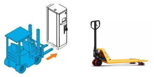
Figure 3-6 handling with forklift
